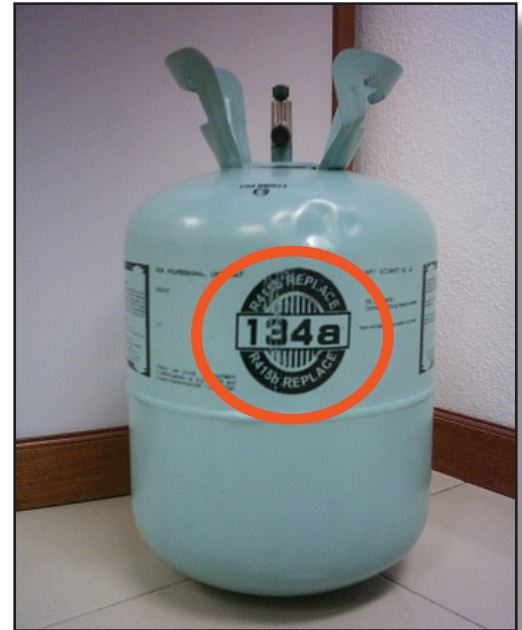
What to look for: R134a is highly visible on the canisters while ‘R415b replace’ is in small, more unnoticeable text surrounding that .
